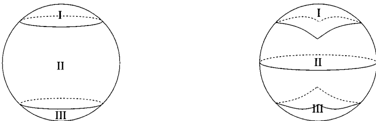
(a) (I) northern hemisphere stereographic projection (II) mercator projection (III) southern hemisphere stereographic projection
